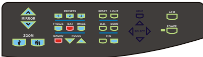
Control panel in "unit on" position, text enhancement and macro function activated - camera menu and help not visible
